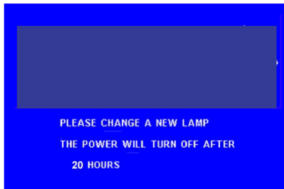
Figure 16 Lamp replacement warning signal
